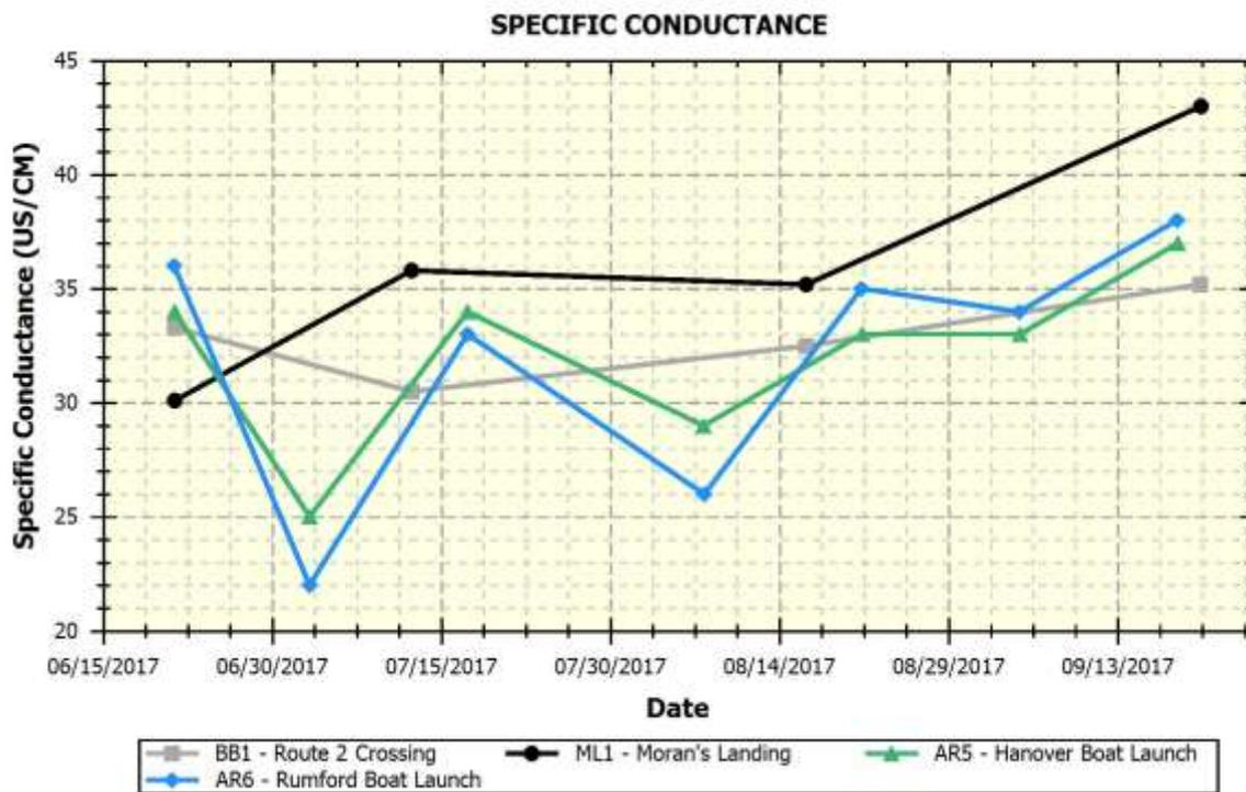
**Figure 5-1-9:** Graph of specific conductance (main stem)
